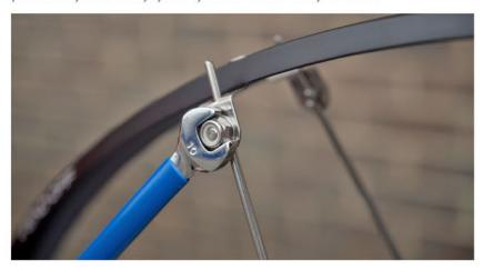
8). Fit the rear wheel and adjust the stays so that the mudguard is aligned with the wheel. Once you are happy with the fit, crimp the rear mudguard bracket with a pair of pliers. Please ensure there is at least a 5mm gap between the mudguard and tyre for debris to pass through.
