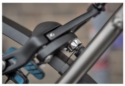
3). If you are running disc brakes and the seat stay bridge hole is near horizontal, mount the rear mudguard bracket using an appropriate nut and bolt. Offer up the rear mudguard to the bracket and carefully fold the bracket around the egde of the mudguard. Do not tighten yet.
