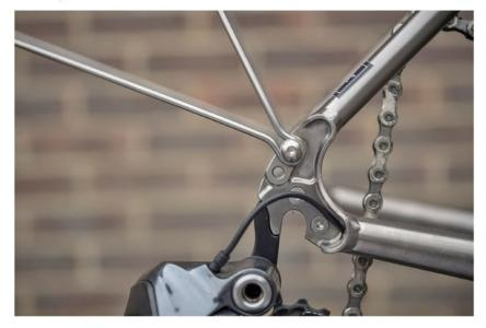
7). Attach the stays to the mudguard using the enclosed eyeletted nut and bolt. If the mudguard eyelets on your frame are located in a high position on your seat stays you may have to bend the stay for best fit
