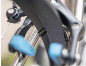
5). Mount the mudguard to your chainstay bridge using the hole provided and an appropriate nut. If you are fitting to a Kinesis RANGE ebike you will need to add a 7mm spacer or stack of washers due to the narrow part of the frame here (see image below). Once the chainstay bridge bolt is tight, return to the mudguard bridge bracket and fully tighten it around the mudguard using pliers wrapped in a rag.
