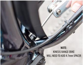
6). Attach the rear stays to the mudguard eyelets on your frame using an appropriate bolt. The eyelets will be located on the dropouts or the seat stays
