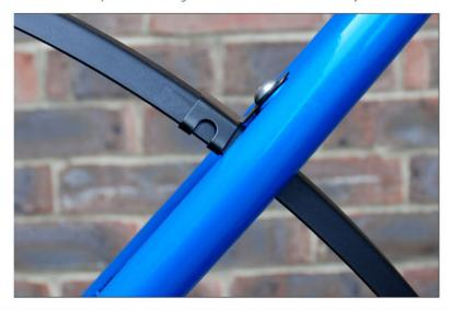
4). If you are running disc brakes and the seat stay bridge hole is underneath, then you will first need to bend the rear mudguard bracket straight. We have reinforced this bracket so you may need to support it in a vice to bend it. Once fitted, offer up the rear mudguard to the bracket and loosely fold the bracket around the edge of the mudguard. Do not fully tighten the bracket fully around the mudguard yet.
