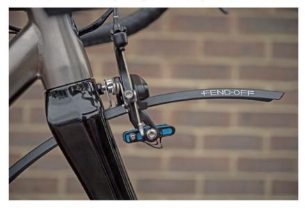
3). If you have a drum or disc brake, mount the bracket to preferably the front side of the fork crown using an appropriate nut and bolt (see below image). Mounting to the rear is fine if this is not possible.
