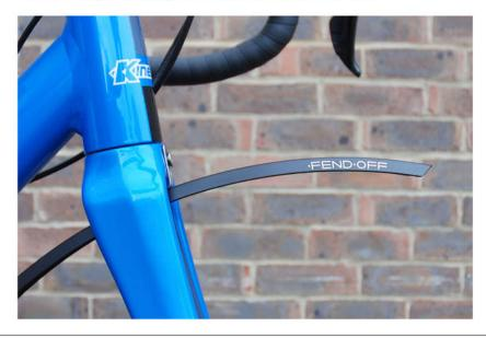
4). Attach the front stays to the mudguard eyelets on your fork using an appropriate bolt. The eyelets will be located on the dropouts or on the inside of the fork legs.
