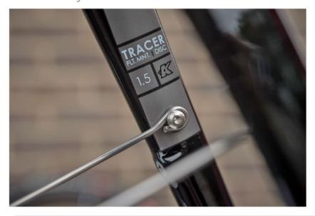
5). Attach the stays to the mudguard using the enclosed eyeletted nut and bolt. If the mudguard eyelets on your fork were located on the inside of the fork leg you may have to bend the stay for best fit
