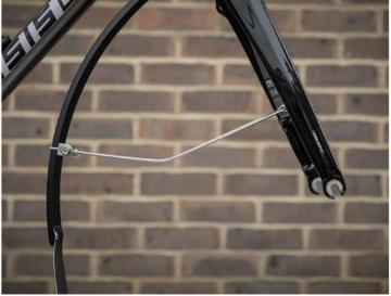
6). Fit the front wheel and adjust the stays so that the mudguard is aligned with the wheel. Please ensure there is at least a 5mm gap between the mudguard and tyre for debris to pass through.
